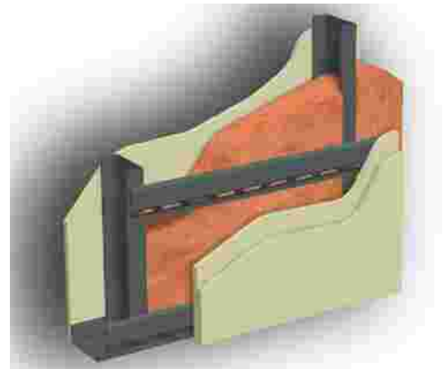
Figure 16: Resilient channels over metal studs break the vibrating path, helping to increase sound transmission loss.
