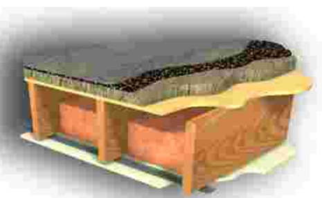
Wood Floors With Various Toppings
